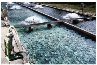
The ejector in the LWS WET system continuously supplies fresh water containing plenty of dissolved oxygen by re-circulating the water in the pond and increasing aerobic bacteria activity.
